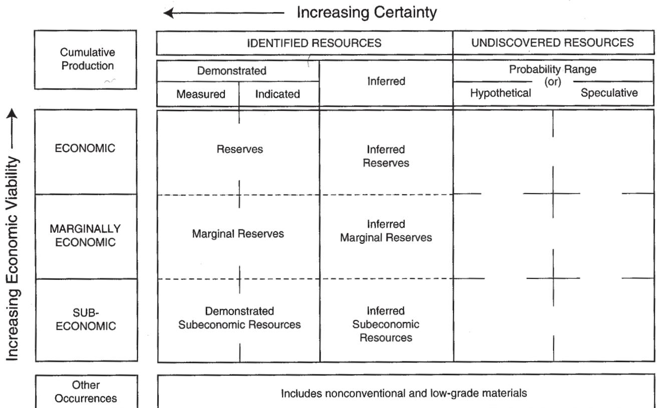
FIGURE 3-1 Classification of Mineral Resources. Source: Mineral Commodities Summaries, U.S. Geological Survey (1992:203)
